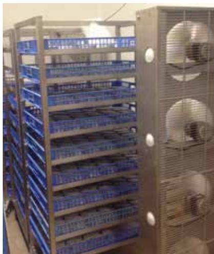
*The sechoir or 'cold drying room' with a bank of fans to increase the evaporation rate.*
