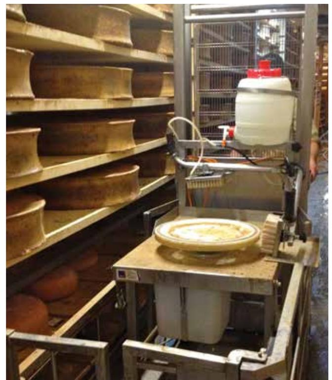
*Top: Brushing Mimolette with a coarse brush. Bottom: The morge is applied to large cheeses using an automated scrubber. As the cheese rotates against the brush, it is kept charged with liquid from the canister above.*
